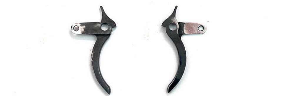
Figure 15: Polished Transfer Bar Holes
